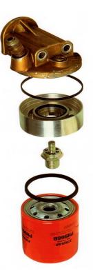
Remove the bolt, bowl, and original filter. Remove the oil seal which sits in the groove in the filter head and clean the groove. Remove the steel boss by inserting a tommy-bar through the hole in the side of the boss and unscrewing it.
